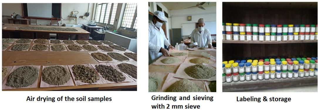
Figure 3: Soil sample preparation and storage
