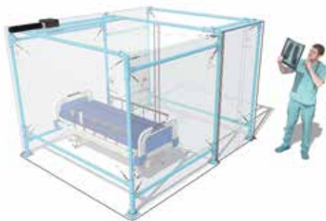
Figure 4: Negative Pressure Cabinet
